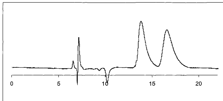
Figure 7.2: Chromatogram obtained using 100% MeOH, 1% TEAA(v/v), 0.4mL/min on Chirobiotic TAG column for separation of racemic hypericin.
